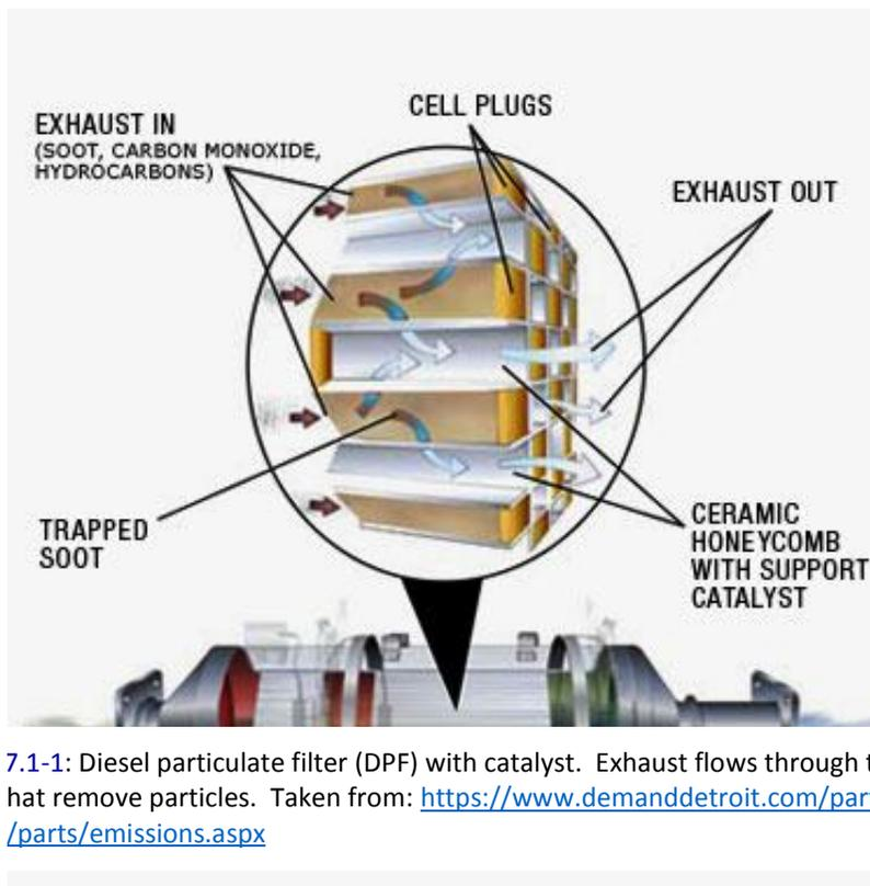
7.1-1: Diesel particulate filter (DPF) with catalyst. Exhaust flows through that remove particles. Taken from: <https://www.demanddetroit.com/parts/emissions.aspx>
