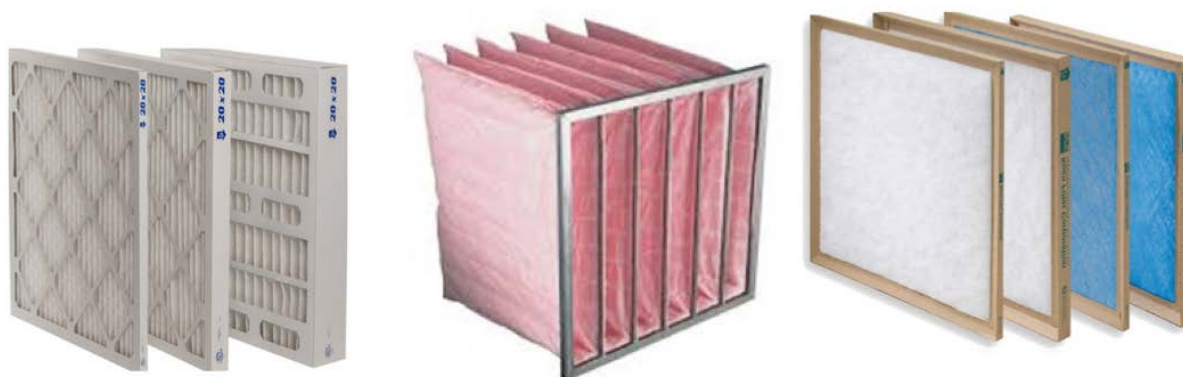
FIGURE 1-1. Examples of filters used in forced air heating/cooling systems and in commercial heating, ventilating and air conditioning (HVAC) systems. Left: extended area filters in three depths with ratings from MERV7 to 13 (high efficiency). Center: Secondary “bag” or “pocket” filter used in commercial HVAC systems. Right: Low cost and inefficient filters often used as furnace filters in homes. Sources: left and right: http://www.qualityfurnacefilters.com/are-pleated-furnace-filters-really-better-than-disposable-fiberglass-filters/ Center: http://www.filtrationgroup.com/WFS/FGCBusiness/en_US/-/USD/HVAC/hvac-pocket-filters ;
