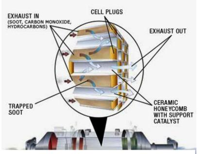
7.1-1: Diesel particulate filter (DPF) with catalyst. Exhaust flows through t hat remove particles. Taken from: <u>https://www.demanddetroit.com/part</u> /parts/emissions.aspx
